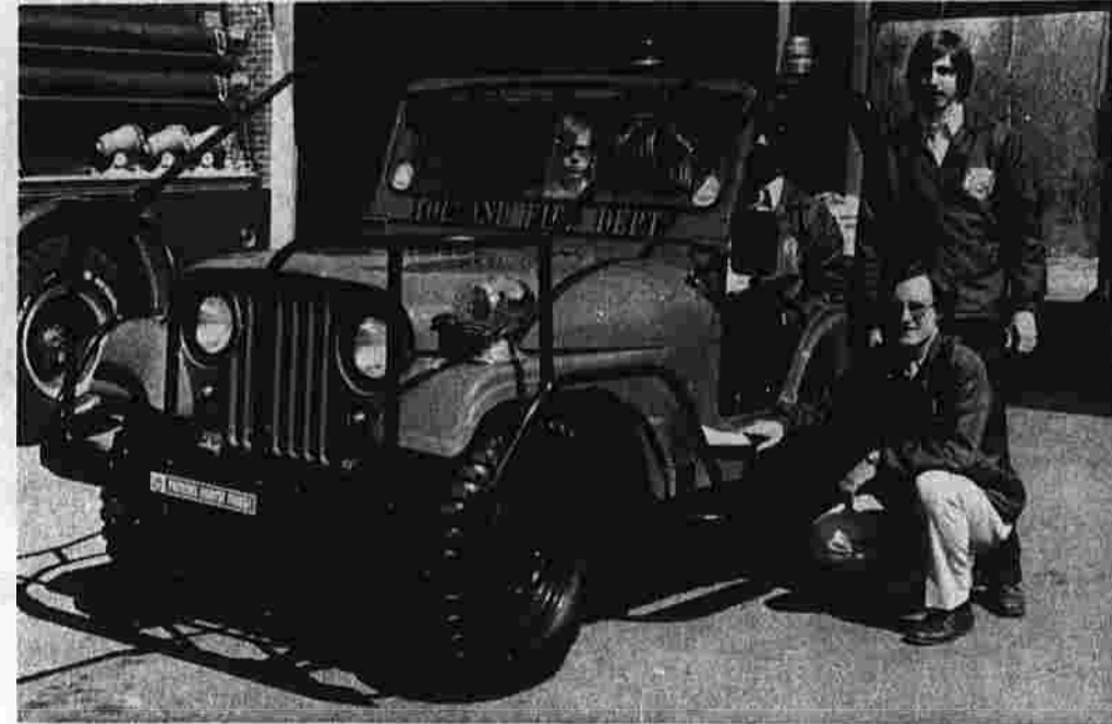
Four members of the Tolland Volunteer Fire Department sit back and enjoy the federal surplus jeep they converted into a jeep pumper to be used for area grass and brush fires and search and rescue operations.
